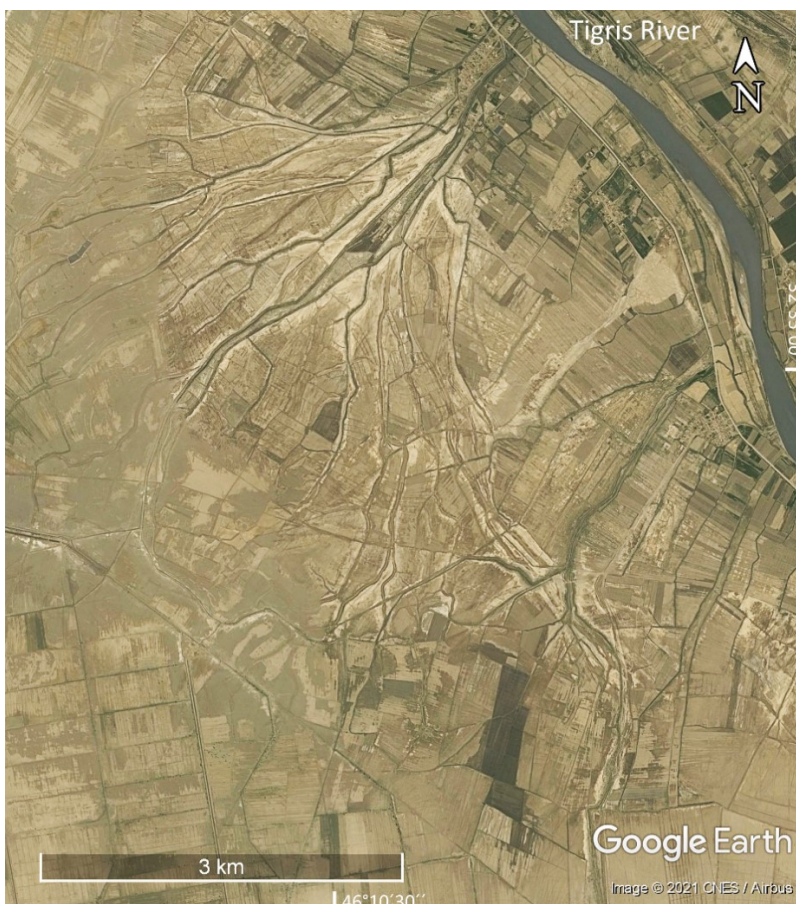
Figure 2: Satellite image displaying fan-like crevasse splays with many active and inactive channels leading water from the River Tigris into its western floodbasins. The curved channels appear natural, the straight channels have been anthropogenically modified.
