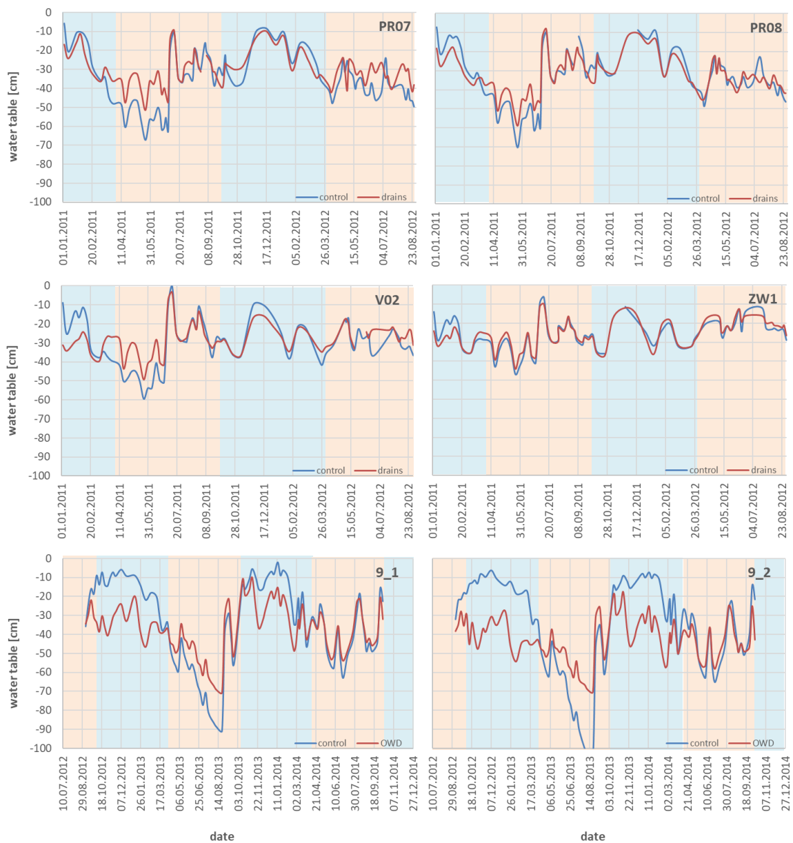
Figure 4: Water table over time measured in plots with (red) and without submerged drains (blue) in parcels in Zegveld (PR07, PR08, VO2, ZW1) and Zeevang (9_1, 9_2). Only the measurements of the sub-parcels with submerged drains at 4 m distance and their control are shown. Blue backgrounds denote winter months, reddish summer. Note the different measurement periods. Data were extracted from Hoving et al. (2013a, b, 2015).
