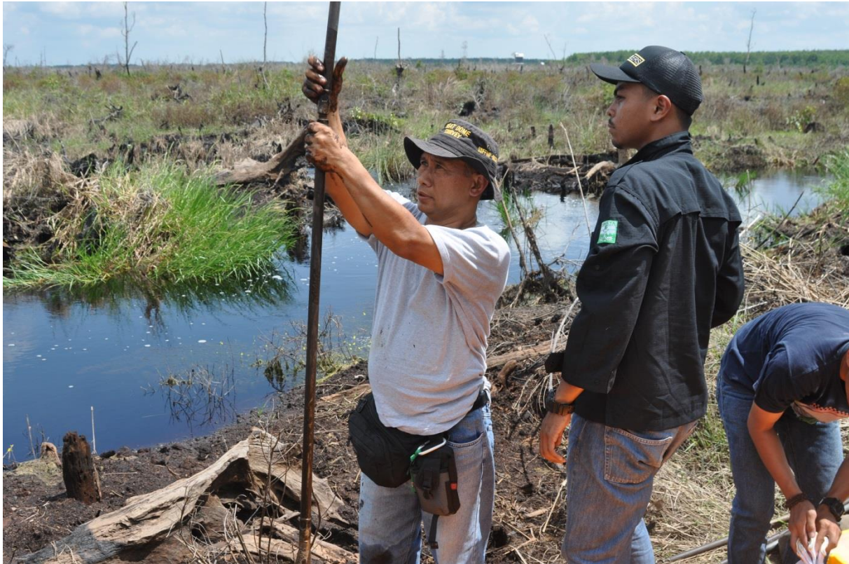
Peat coring in Sumatra with dr. Muh Bambang Prayitno, Sriwijaya University, Palembang. Photo: Hans Joosten.
