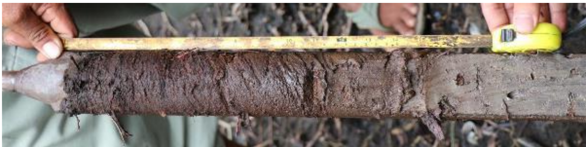
Typical peat sample with underlying marine clay layer
